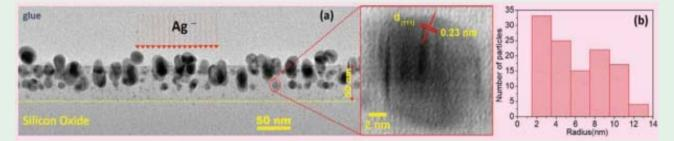
(a) The-cross sectional TEM image of the silver implanted SiO2 film/Si (100). The red arrows show the direction of silver ion implantation. Towards the right, the high resolution image shows the single crystalline nature of the formed Ag nanoparticles. (b) The corresponding size distribution of the Ag nanoparticles. (*Fig. of Sec-E*)
