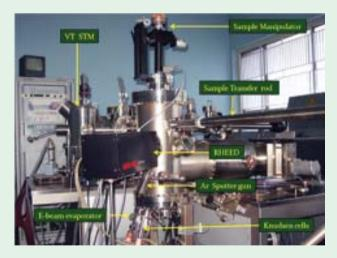
pressures (ultra high vacuum, UHV conditions) and appropriate cleaning of surfaces. The Molecular Beam Epitaxy (MBE) – Variable Temperature Scanning Tunneling Microscope (VTSTM) system is a custom designed unit procured from M/S Omicron GmBH, Germany. The facility consists of three Knudsen cells, one
