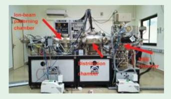
integrated with molecular beam epitaxy system for fabrication of self-organized patterned susbstrates, *in-situ* ultrathin films and selfassembled nanostructures to achieve nanoscale functionalities, viz. plasmonics, magnetism and optical properties. This facility is having structural characterization module and we are in the process of adding the in-situ compositional module as well which will make it a unique system in the country.
