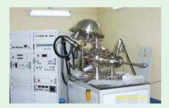
The present XPS system has a dual X-ray Aode (Mg/Al). The sample can be aligned by a manipulator. Photoelectrons are energy analyzed by a hemispherical mirror analyzer. The system also has the facility for sample annealing and Ar ion sputtering. Sputtering technique can be utilized for doing depth profiling studies. All the experiments are carried out under ultra high vacuum (UHV) conditions at the vacuum of 1x10-10 Torr.
