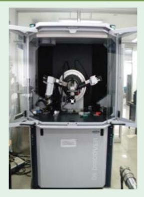
quantitative phase identification, crystal structure identification of different samples, X-ray reflectivities crystallite size determination, strain analysis and preferred orientation for established structures. In addition, we have another XRD Setup (D8, Advance), which is also in operation.
