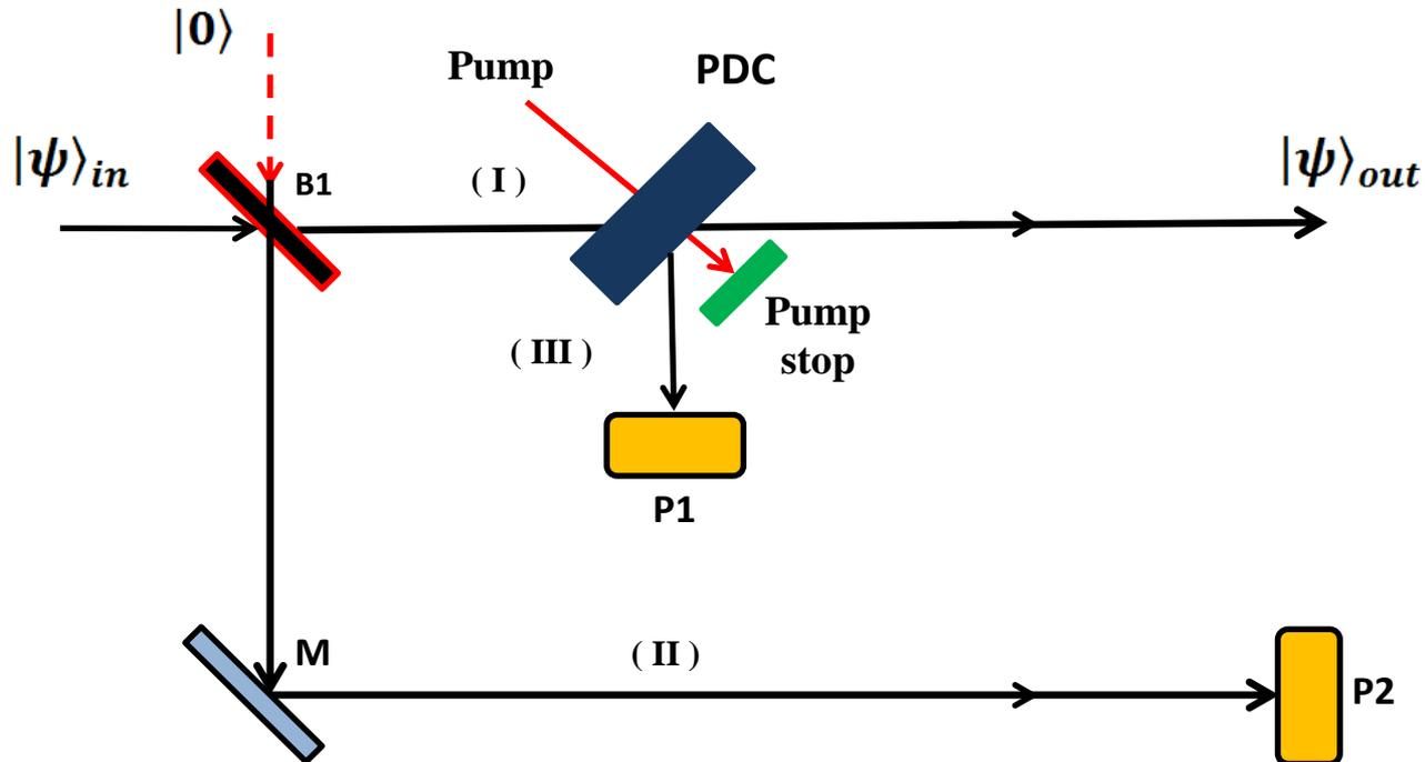
Photon detection at **P1** and **P2** ensures that the operation  $\hat{a} \hat{a}^\dagger$  has been performed with some probability. **M** is a highly reflective, lossless mirror.
