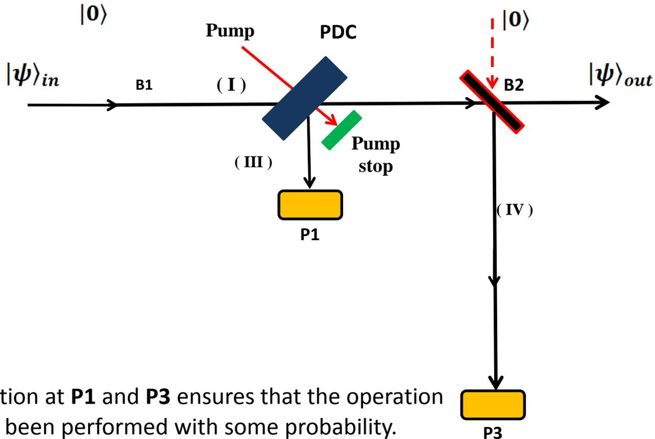
Photon detection at **P1** and **P3** ensures that the operation  $\hat{a}^\dagger \hat{a}$  has been performed with some probability.
