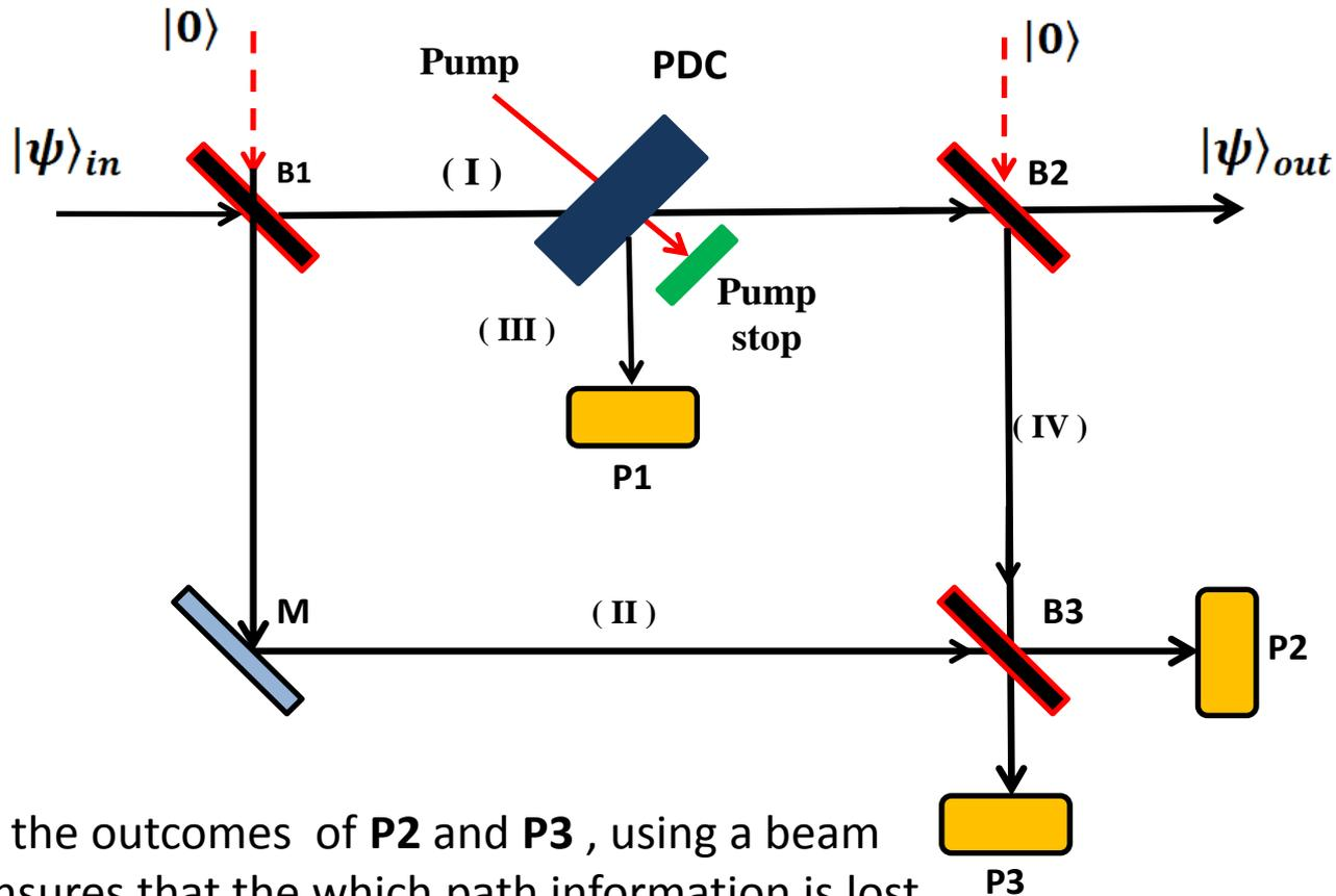
Interfering the outcomes of **P2** and **P3**, using a beam splitter **B3**, ensures that the which path information is lost and we have the operation  $s\hat{a}\hat{a}^\dagger + t\hat{a}^\dagger\hat{a}$ .
