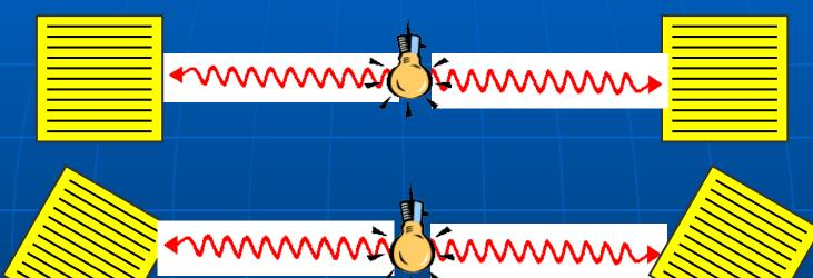
If one photon passes through the polaroid, so does the other one. Therefore each photon must already have its instructions about what to do when it meets the polaroid.
