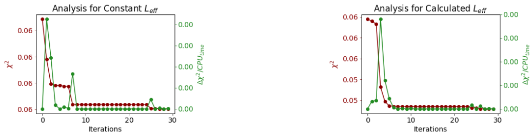
Figure 3. Plot showing \chi^2 values and \Delta\chi^2/CPU_{time} plotted against the number of fitting iterations for constant and calculated L_{eff} respectively.
