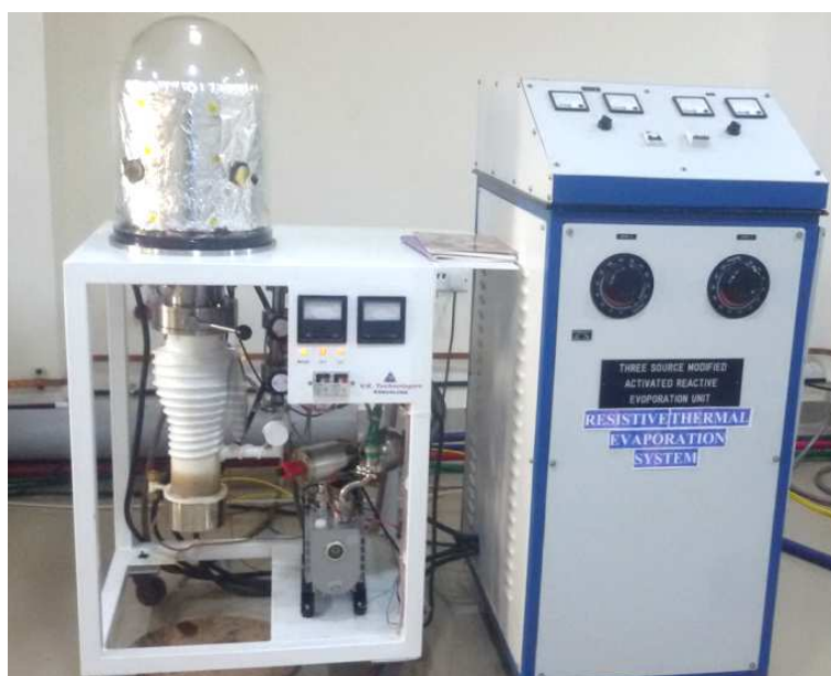
Figure 2. Resistive thermal evaporation unit for deposition of Al thin films
