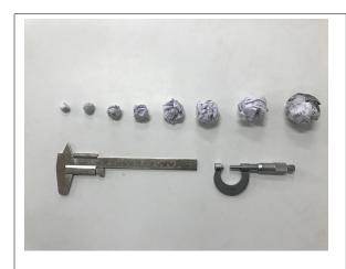
**Figure 1.** Measuring the diameter of crumpled paper balls
