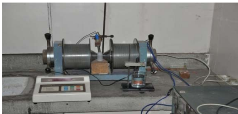
Figure 3. Experimental setup of electromagnets for measurement of pH of distilled water
