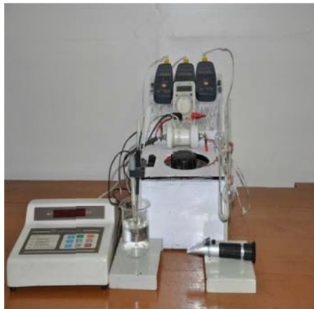
Figure 1. Pictorial representation of ohmic heating system
