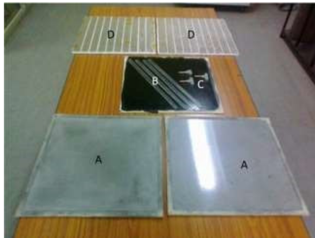
Figure 1. Various components for RPC fabrication. Two graphite coated bakelite sheets (A), edge spacers (B), gas nozzles (C) and pick-up strips (D).
