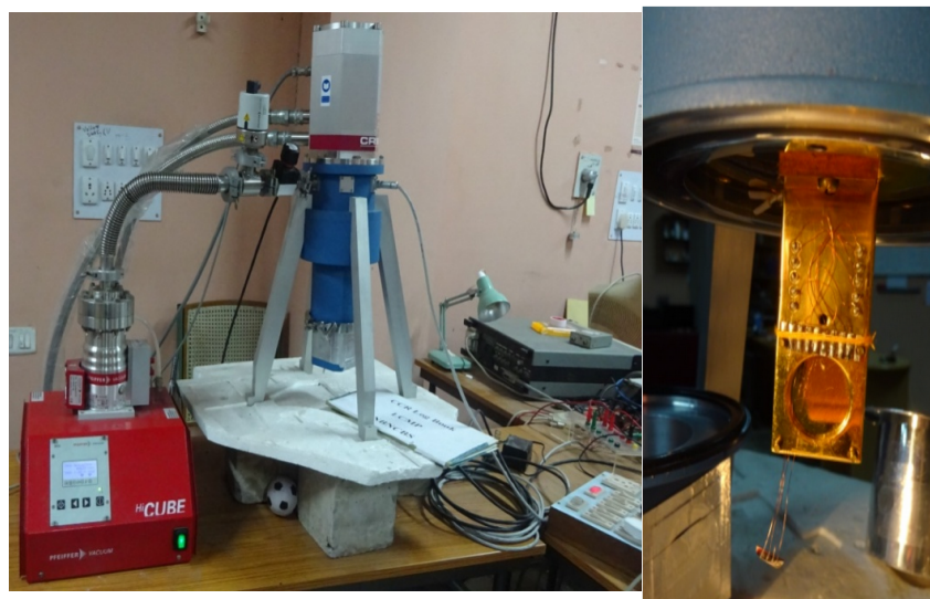
Figure 3. Indigenously designed set up to measure resistivity using ac four probe method
